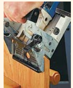
▲ Many plate joiner fences adjust to trap the point of a 45° bevel.
