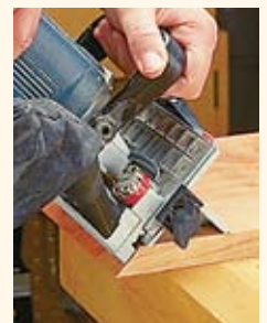
▲ Some plate joiner fences adjust to fit over the inside corner of a 45° bevel.
