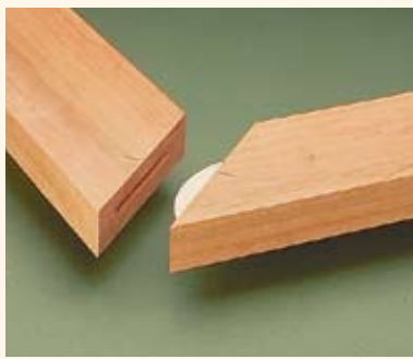
▲ Adding a biscuit to the ends of mitered pieces is a quick way to strengthen a frame.
