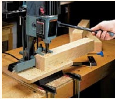
▲ Mortising Machine. Hollow chisels drill out the mortise and square up the ends all at once.
