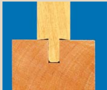
▲ Perfect Fit. To get a tight joint-line, undercut the shoulders of the tenon with a chisel.
