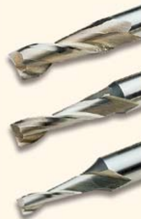
▲ The deep flutes of a spiral end mill bit are designed to pull the shavings out of a mortise quickly.
