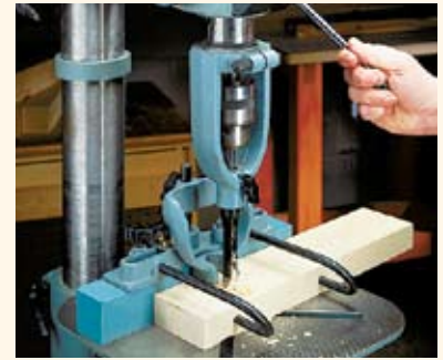
▲ Mortising Attachment. Mounted on a drill press, this attachment works like a mortising machine.
