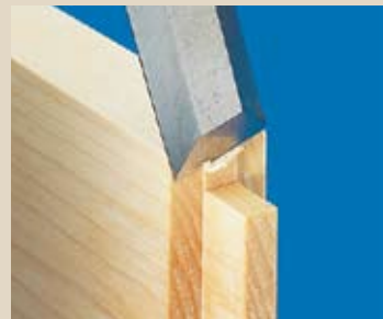
▲ Stepped Shoulders. Cut shoulders on edges of tenon slightly proud, then trim flush.
