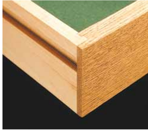
Flush Joint. Grooves in the sides of the drawer recess the guides that it runs on. So the front is flush with the sides.
