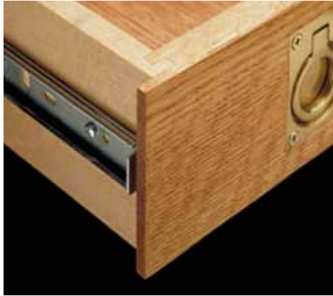
Lipped Joint. To hide the metal slides, this locking rabbet has a lip on the drawer front that extends past the sides.
