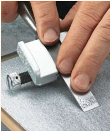
▲ Long, back-and-forth strokes with firm pressure on the tip will quickly flatten the bevel and remove nicks.
