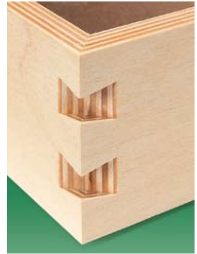
Cut Slots. The jig positions the project securely to cut a dovetail-shaped slot for a key.
