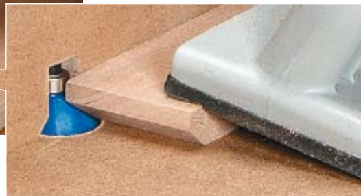
▲ Seamless Surface. An auxiliary tabletop made from 1/4" hardboard creates a smooth, zero-clearance worksurface around the router bit (inset photo).
