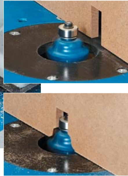
▲ Custom Face. Pivot the fence into the bearing on the bit to create a zero-clearance opening, simply pivot the fence into the spinning bit (inset photos above). Since only a small part of the bit is exposed, the workpiece will always be fully supported.
