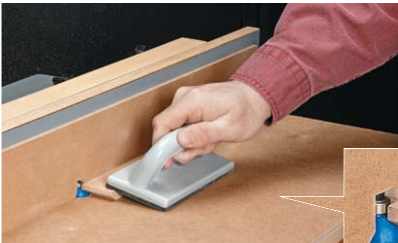
▲ Seamless Surface. An auxiliary tabletop made from 1/4" hardboard creates a smooth, zero-clearance worksurface around the router bit (inset photo).
