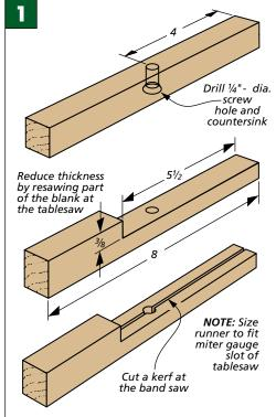
After drilling a countersunk hole on the underside for the machine screw, you can cut the runner to form the shoulder, you can. Finally, cut a kerf down the center. This allows the runner to expand when under pressure from the tapered head of the screw, locking it in position.
