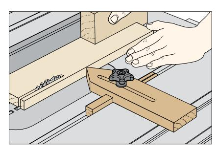
When it comes to cutting strips thinner than ½", the conventional method of setting the rip fence for the width of the cut isn't always the safest method. Trapping the thin strip between the fence and the blade can result in the workpiece being kicked back at high speed. But moving the fence between cuts so the strip falls to the outside of the blade requires tedious measuring. It's also tough to maintain a consistent thickness of the strips. A safer
