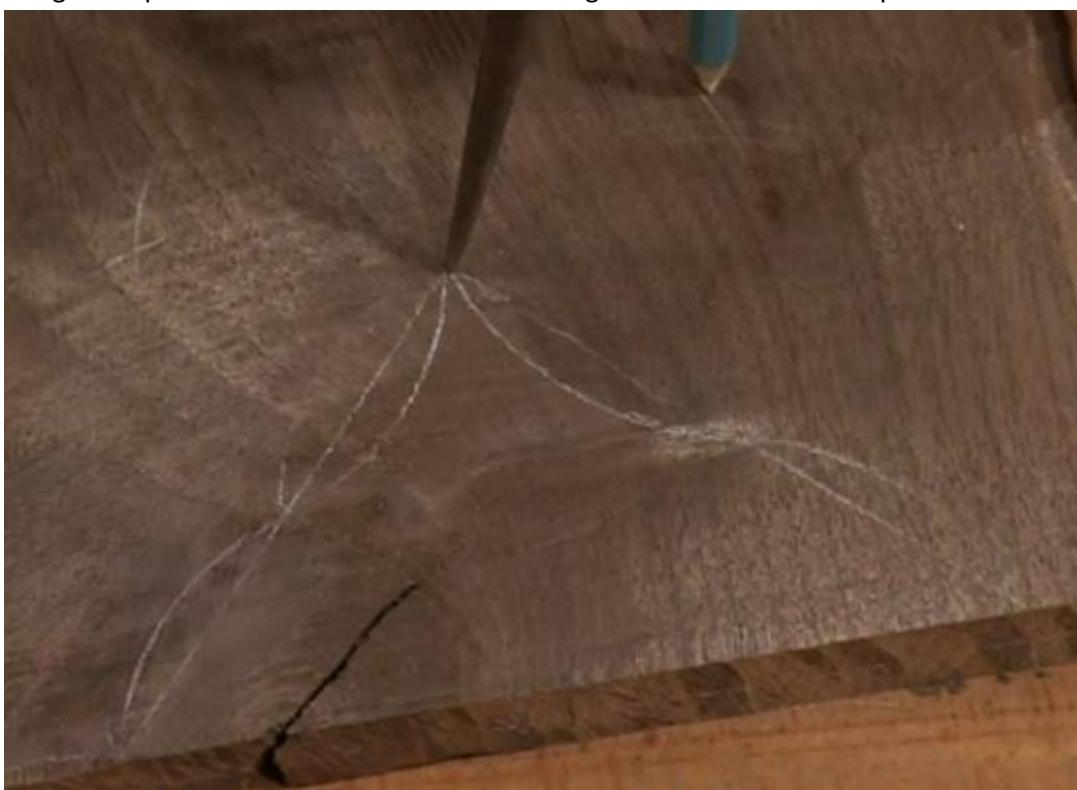
Draw an arc from one end of the half line and another from the center to make an intersection. Use the new intersection to draw each arc of the ogee. Use a scrap block to anchor the compass for the lowest arcs. Cut it out with a coping saw.
