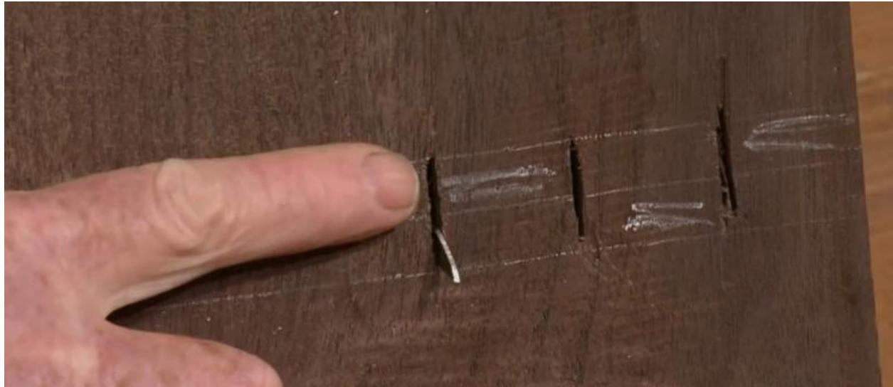
Press the tip into the hole and pull with short strokes until the cut is long enough to use a thin keyhole saw blade to finish the cut to the lines on both sides. These have to be very precise as they are the knuckle edges.
