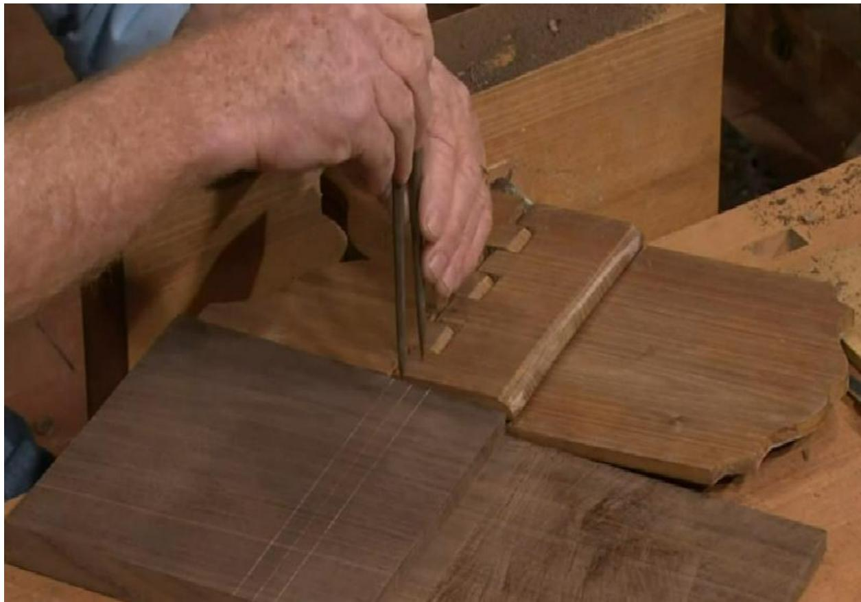
Using the lines on the circles as a guide draw 3 lines across the face and back sides. With a divider pace off an ODD number for the joints. 3 or 5 works for smaller pieces and 7 - 9 for wider stock;
