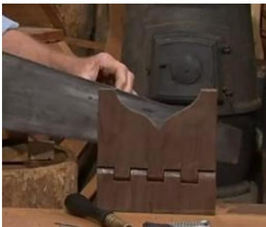
Place the work piece into a bench vise and use a sharp hand saw (or a bow saw, cutting on the push stroke) to cut down the centerline, turning your piece around often to stay true on both sides. Let the saw do the work so it does not bow inside of the cut and snap or damage the final work.
