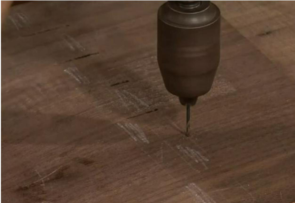
Carefully mark the areas to be cut out. When laying out, using a drill really helps to keep both sides the same. Using a 1/16<sup>th</sup> bit, drill completely through at each corner of the knuckle. The hole will guide the tip of the blade all the way through the work piece.
