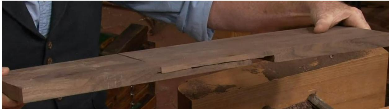
Notice that the first cut is at about 10" for the back and a notch between the two pieces. They are cut apart when sawn with a bow saw down the length creating two pieces.
