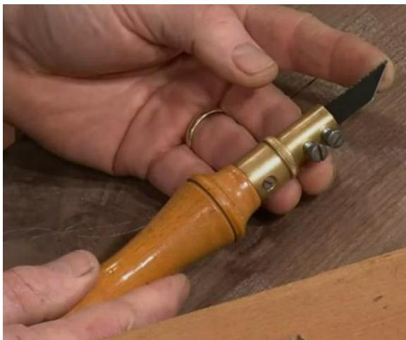
Using a pad saw with a hack saw blade (mounted backward so it cuts on the pull stroke) insert the tip into the hole and pull back to cut the joints completely through the piece without going over the line on either side.
