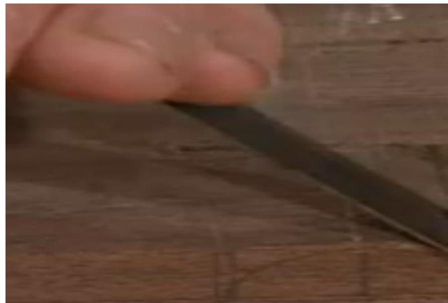
As the cut takes shape use a thin paring chisel to clear out the remaining wood, staying to the outside of the line.
