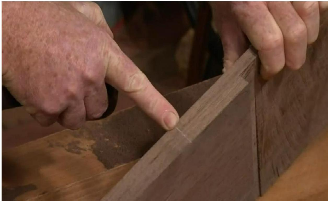
Use a marking gauge set at  $\frac{1}{2}$  the width of the wood to draw a line down the entire center of the thickness on both sides.
