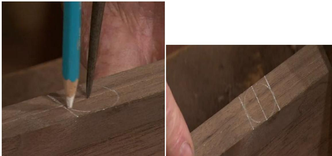
Using a compass set at  $\frac{1}{2}$  the thickness of the wood, scribe a circle above the line on both sides and draw lines across the top, bottom and center of the circle to create the knuckle joint;
