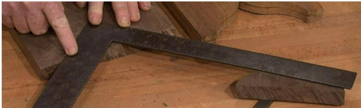
Lay a square so the point is in the center of the work piece and the 4" on each leg match left to right at the bottom.
