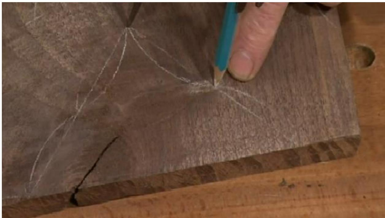
Using a compass set at half the distance of one leg mark the center and repeat on the other leg.
