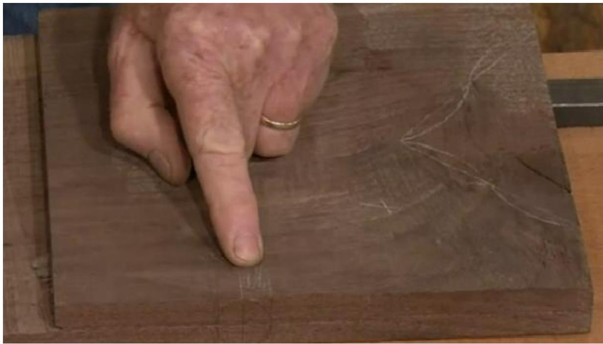
Before using a chisel to remove the wood marked for removal, make sure the work piece is flat on the bench. Use a firmer chisel to make a cut straight down and follow up with an angle cut, working your way down.
