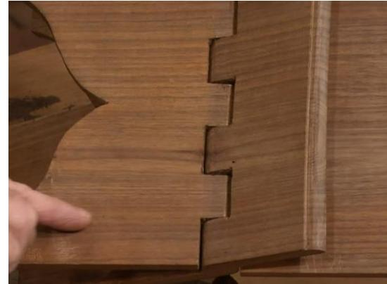
Make sure that the short section is continuous so the piece doesn't split;
