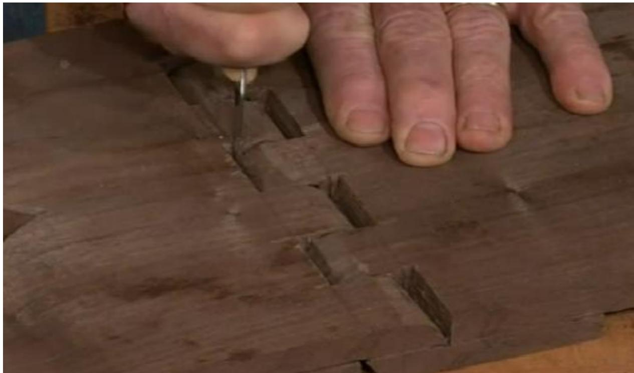
Use a knife to carefully open up the last remaining wood between the knuckles to open the bookstand. Smooth it up with a plane or light sanding.
