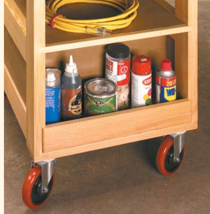
▲ Storage Cubby. Adding a false front to the opening at the back of the cart creates a handy storage area for often-used items.
