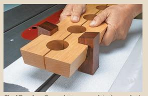
**Final Touches.** To get the bottoms of the feet perfectly flat, use some adhesive-backed, 120-grit sandpaper on a flat surface, like your table saw.
