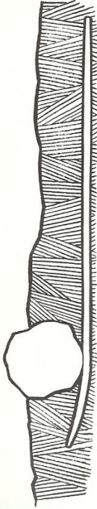
Figure 5: One method for shaping batten.
