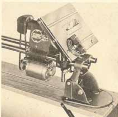
Bevels and miters are cut by using the miter gauge, tilting the table, or both.
