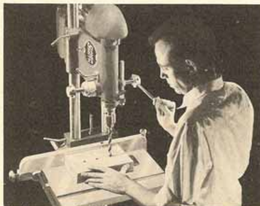
Rip fence — standard equipment — serves as guide for accurate parallel drilling.
