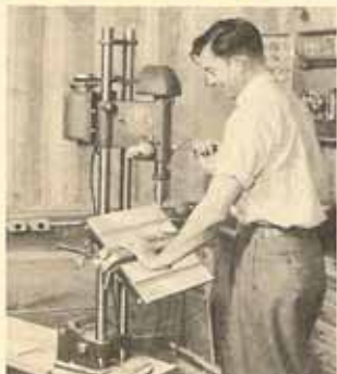
Fence and tilting table quickly form "V" block to make angle drilling easy and accurate — handy for dowels, rods, pipe, etc.
