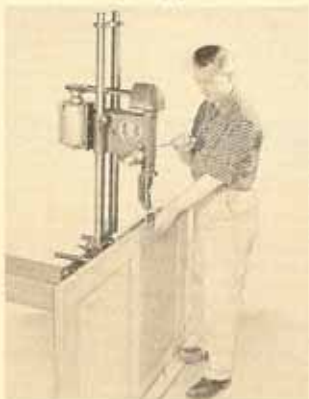
Fence and tilting table quickly form "V" block to make angle drilling easy and accurate — handy for dowels, rods, pipe, etc.
