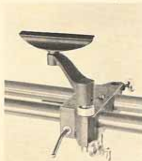
Parallel movement of the carriage and versatile adjustment of the tool rest are superior features.
