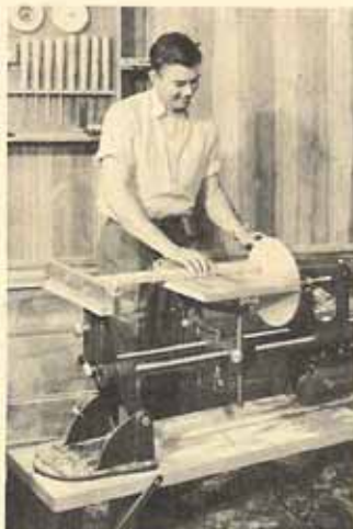
Only with SHOPSMITH can disc be fed against workpiece for fast and accurate duplicate sanding.
