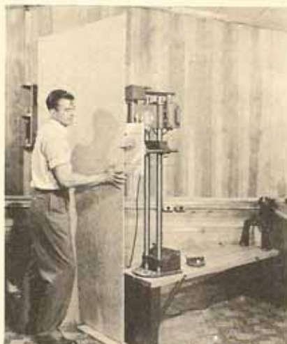
Large workpieces can be handled in an upright position with the vertical saw — a unique SHOPSMITH feature.
