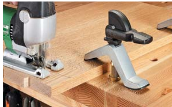
◀ Hold-Downs. These cam-activated hold-downs secure a workpiece and allow you to reposition it quickly.
