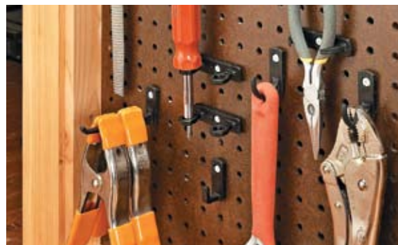
◀ Hooks. Reinforced plastic hooks lock into the pegboard so you never have to worry about them falling out.
