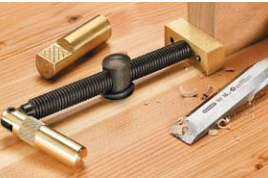
◀ Clamping. A round brass bench pup and a threaded Wonder Pup create a handy "bench vise."
