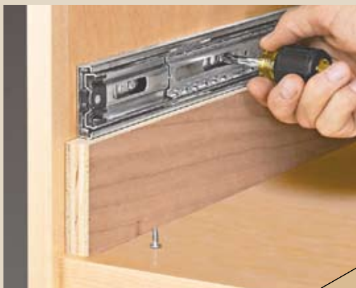
▲ Installing Slides. A scrap of plywood makes it easy to level a drawer slide in the case. Center the other half of the slide on the drawer side (right).
