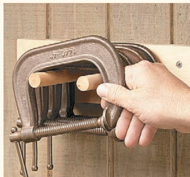
▲ C-clamps are held on this simple rack. It can be custom built to fit different sizes of clamps.
