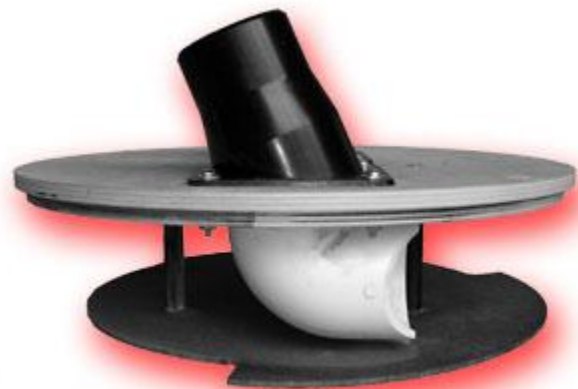
Another view of the guts showing the relationship of the elbow to the baffle's expanded (120-degree) section. Testing indicated that this design minimized turbulence.
