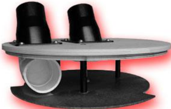
The guts of the lid. The elbow was slightly modified so it can sit flush to the top of the lid and so it can hug the side of the can a little.
