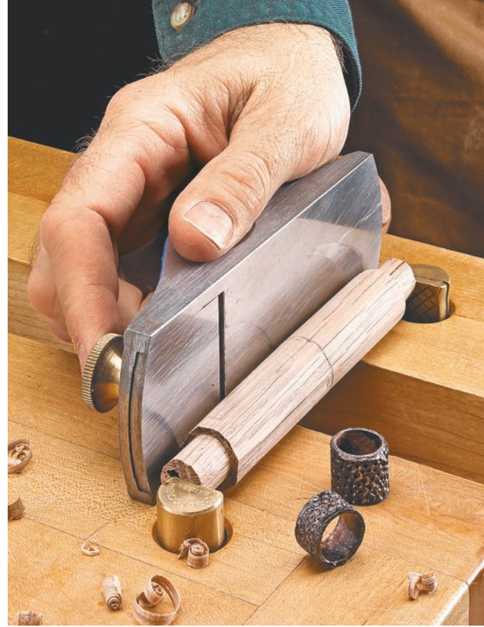
▲ The Final Touch. Starting from the center, taper the handle toward both ends using a block plane to create a faceted, barrel shape.
