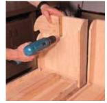
wing is to attach the hinge to the upright assembly. Then remove it. and attach it to the wing. Clamp the upright in a vise and reattach everything. Make sure to mark each hinge's location. Otherwise you'll mess up how some parts go together.
