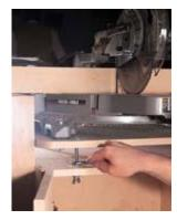
easy as loosening the wing nuts inside the cabinet and using the jam nuts on top of the cabinet to raise or lower the saw until it's flush with the wing assemblies.
