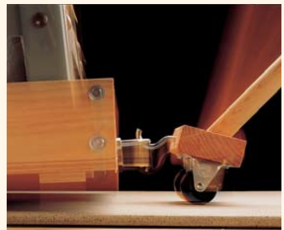
▲ Easy Lifting. Leverage and this simple hardware hitch (consisting of a U-bolt and a screw hook) are all that's required to lift a heavy power tool and maneuver it around when you're in a tight space.
