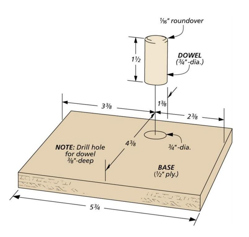
This easy-to-adjust bench dog is nothing more than a square piece of plywood with a dowel inserted in a hole in the face of the piece. The key to the bench dog's adjustability is that the dowel is placed in an offset position from center.
