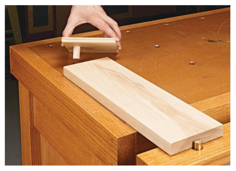
The woodworking vise on my workbench doesn't have a quick-release feature. This can make it a little slow to adjust. To speed up the process when securing a workpiece using bench dogs, I came up with the simple accessory shown above. It allows me to hold a workpiece between it and a unique bench dog inserted in the vise with a minimal amount of adjustment.
