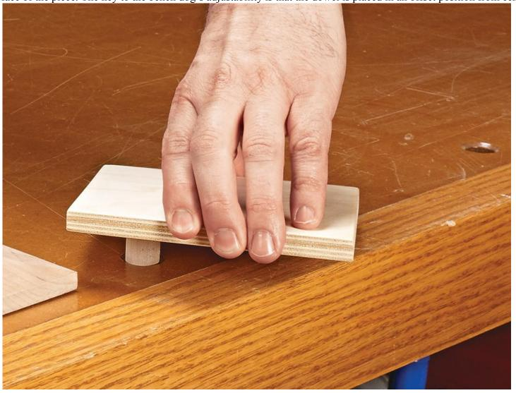
This way, by simply rotating it in the dog hole from one edge to the next, the distance from the workpiece changes as well (4", 3", 2", 1"). This reduces the number of turns of the vise handle needed to secure the piece.
