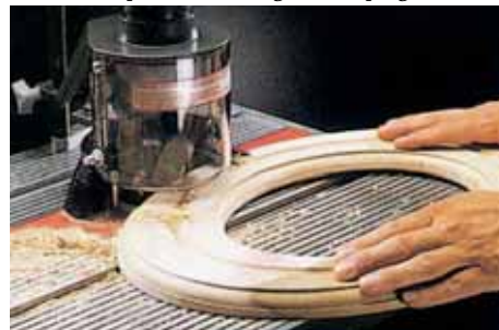
The see-through Shield protects your eyes from flying chips and helps you collect the dust before it becomes a problem.
